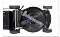
• The mulching blade supplied as standard and the streamlined deck ensure optimal cutting efficiency and perfect feed to the grass catcher.
