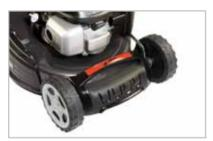
Front bumper with integrated carry handle (B&S and Honda models) providing greater protection of the deck against accidental impact.
