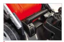
• Centralised cutting height adjustment device controlled by a rugged and ergonomic handle: provides 5 different height positions that can be selected easily and effortlessly from a minimum of 28 mm to a maximum of 75 mm
